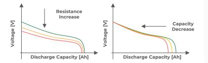
During the degradation process, the resistance of the battery may increase while its capacity decreases. Both of these factors contribute to a decrease in the discharged capacity, which may result in being lower than the nominal capacity (in green), as illustrated on the left, where the effects of the two factors are represented individually.
